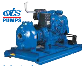
O Series® Engine driven Size: 4" (100 mm) Power: Deutz - Diesel Max Capacity: 730 GPM (46.1 lps) Max Head: 280' (85.3 m) Materials of Construction: Copper Alloy, Aluminum or Steel Impeller, Ductile Iron or Cast Steel Housing
