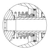
**SEAL DETAIL** Mechanical, Oil Lubricated, Double Floating, Self-Aligninig. Tungsten Titanium Carbide Rotating and Stationary Faces and Stainless Steel 316 Stationary Seat. Fluorocarbon Elastomers (DuPont Viton® or Equivalent). Stainless Steel 303/304 Cage and Spring. Maximum Temperature of Liquid Pumped, 160°F (71°C).\*
