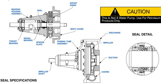
Seal: Mechanical; Self-Lubricated. Fluorocarbon Elastomers (DuPont Viton® or Equivalent). Carbon Rotating Face; Ni-Resist Stationary Face; Maximum Temperature of Liquid Pumped is 160°F (71°C).\*
