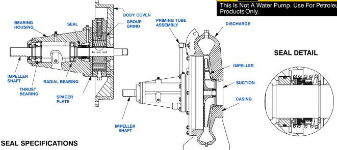
Seal: Mechanical; Self-Lubricated. Fluorocarbon Elastomers (DuPont Viton® or Equivalent). Carbon Rotating Face; Ni-Resist Stationary Face; Maximum Temperature of Liquid Pumped is 160°F (71°C).
