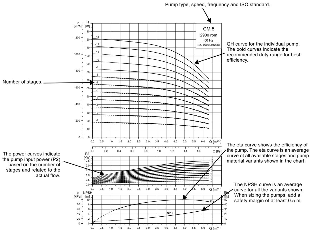
Fig. 34 How to read the curve charts
