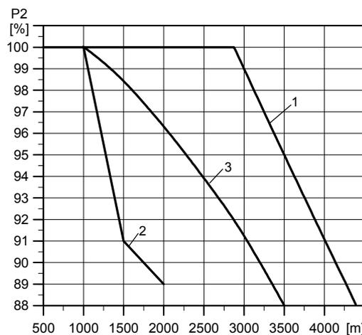
**Fig. 10** Relationship between motor output (P<sub>2</sub>) and altitude
