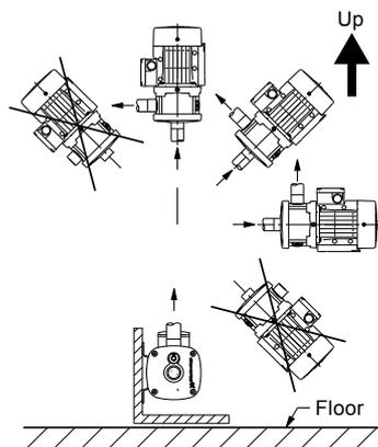
Fig. 11 Positions of CM and CME pumps
