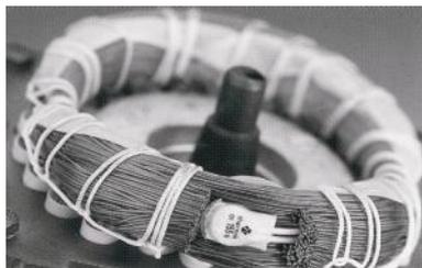
Fig. 46 Thermal switch incorporated in windings
