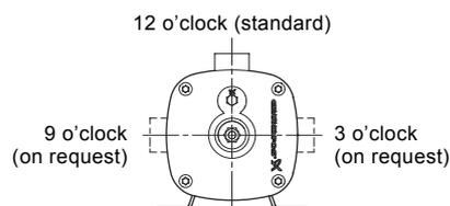
**Fig. 49** Alternative connection positions as seen from pump inlet side
