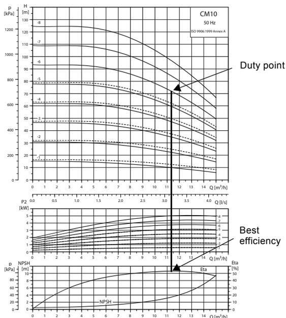
Fig. 32 Example of a CM pump's duty point
