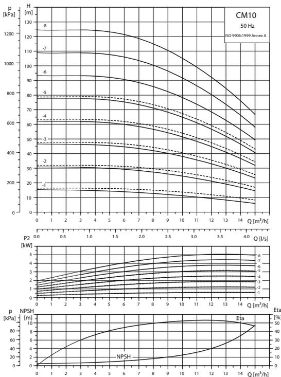
Fig. 29 Example of a curve chart
