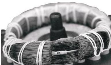
**Fig. 44** PTC sensor incorporated in windings
