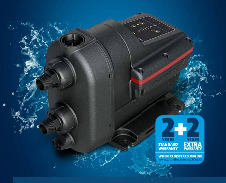
**GRUNDFOS SCALA2** is a robust, composite, variable speed pump that adjusts performance according to water demand, providing constant pressure to all taps. The fully integrated pump includes a motor, tank, sensor, drive and non-return valve in one compact unit that is quick and easy to install. SCALA2 is self-priming, allowing for use from both above and below ground water sources and the water-cooled motor ensures quiet operation.
