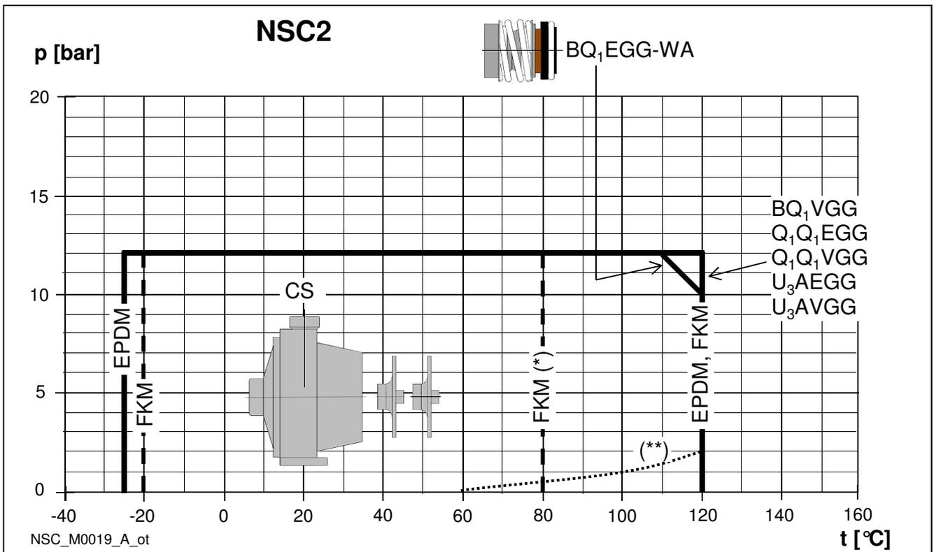
(\*) hot water (\*\*) minimum pressure required at mechanical seal (hot water; could be different in case of other liquids).
