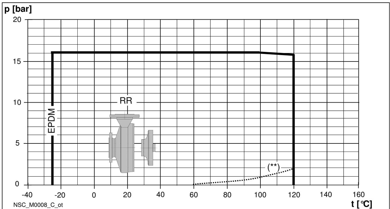
(\*\*) minimum pressure required at mechanical seal (hot water; could be different in case of other liquids).
