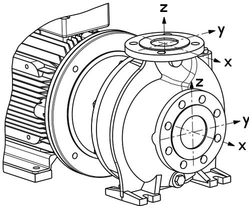
Forces at the pump flanges calculated according to EN ISO 5199:2002.
