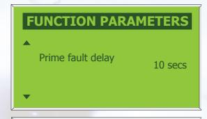
If selected, this parameter enables the operator to set the time value, after which time a prime loss, or flow loss alarm is triggered. This feature is enabled by way of the 'Mode' DIP Switches
