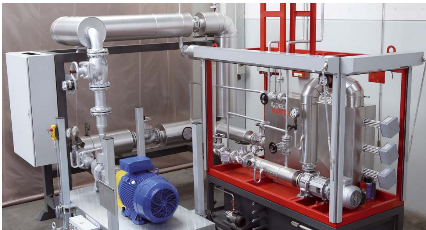
Thermal oil test stand with pump surveillance system on the premises of Speck in Roth. Research of impacts of high temperatures up to 350 °C on the lifetime of the pumps.
