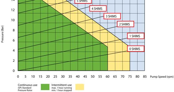
For product temperatures above 65°C and/or viscocity above 2000 mPas use one shim less than shown
