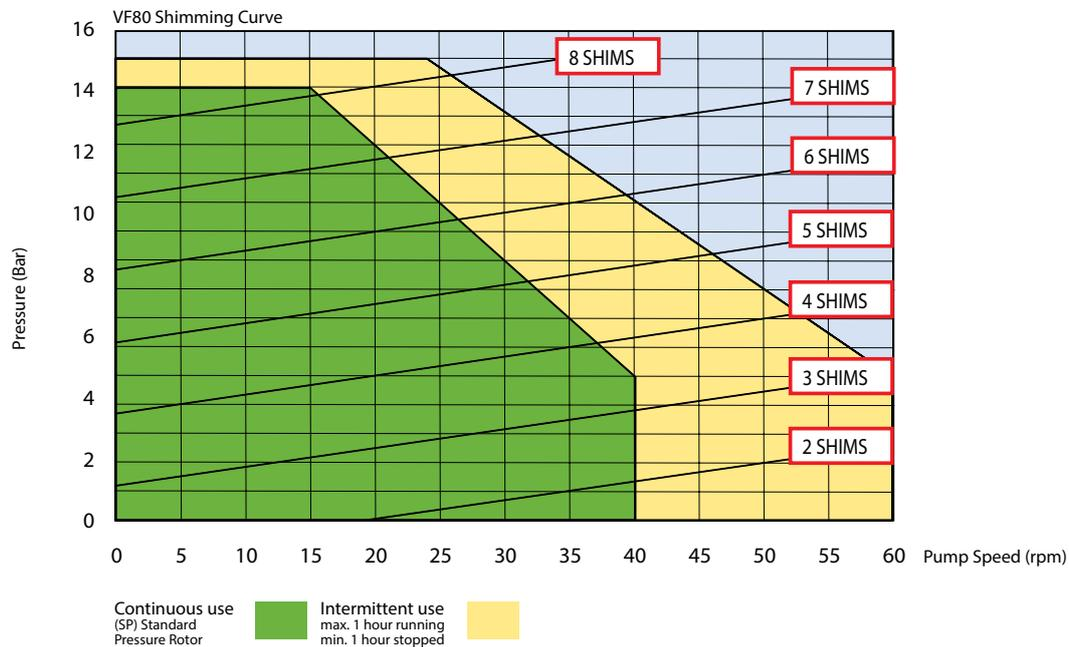
For product temperatures above 65°C and/or viscosity above 2000 mPas use one shim less than shown
