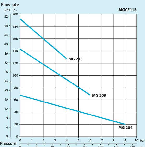
Note: Characteristics with water at 20 °C (68 F) and without relief valve, max vacuum 724 mmHg. Use filter before pump inlet not larger than 10 micron. Unit weight: 1.1 kg (2.4 Lb). Temperature requirements different from ambient temperature must be mentioned on the order.
