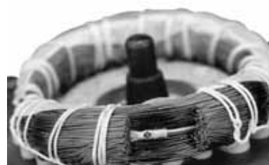
Fig. 24 PTC sensor incorporated in winding
