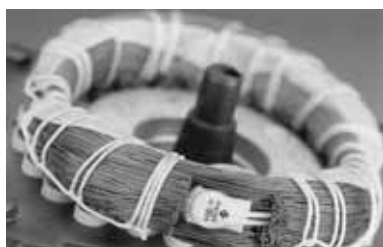
Fig. 26 Thermal switch incorporated in winding
