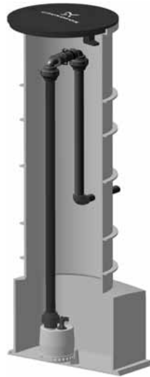
Fig. 13 Pit with free-standing pump with goose neck outlet
