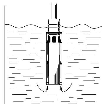
**Fig. 34** Flow sleeve function
