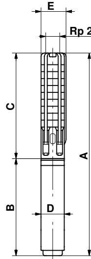
SP 9-56 to SP 9-86 are mounted in sleeve for R 2 connection.
