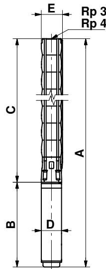
SP 60-24 to SP 60-30 are mounted in sleeve for R4 connection
