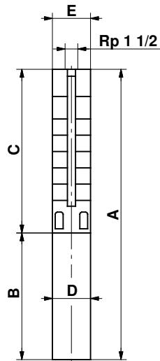
SP 5A-75 and SP 5A-85 are mounted in sleeve for R 1 1/2 connection.
