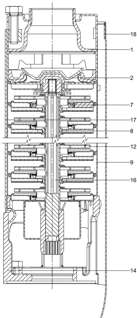
Fig. 8 Example SP3A, pump with spline shaft.
