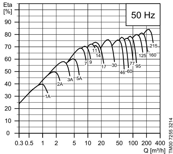
Fig. 1 Pump/motor efficiencies in relation to flow
