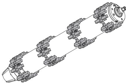
**Fig. 32** Submersible motor fitted with anode strings
