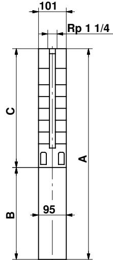
101 mm = Maximum diameter of pump inclusive of cable guard and motor.
